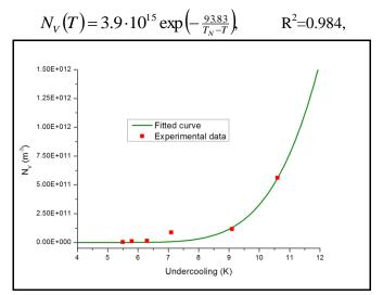
Fig. 6. N<sub>v</sub> on undercooling dependence for  $40 \mu m$  particles.
