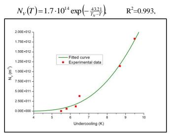
Fig. 5.  $N_V$  on undercooling dependence for <u>10 µm</u> particles.
