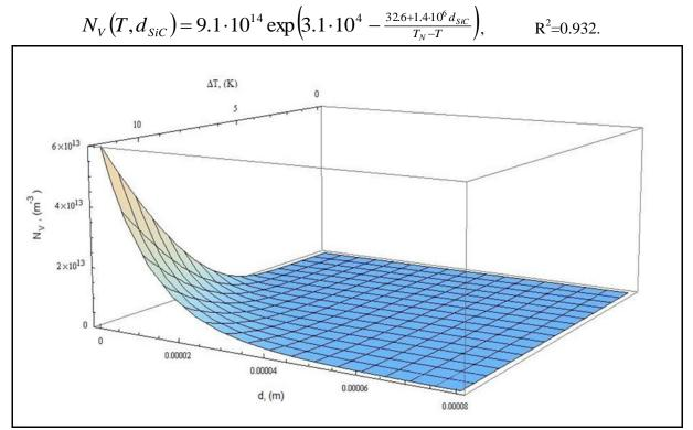
Fig. 8. N<sub>v</sub> dependence on undercooling and mean grain diameter.
