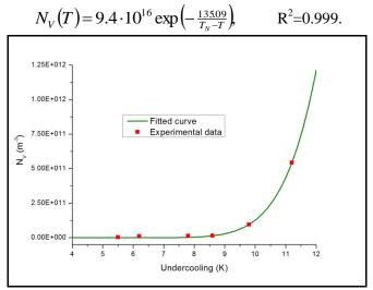
Fig. 7.  $N_V$  on undercooling dependence for <u>76  $\mu$ m</u> particles.
