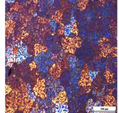
Fig. 2. 2% of SiC, particles mean diameter 40 µm;
